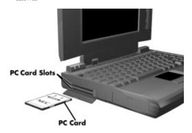
Inserting a PC card
