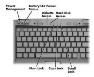
**Power Management** — Green when On; no color when Off; blinking green when the system is in Suspend mode.
