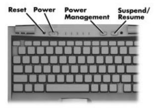
**Reset** — This recessed switch resets the system if the NEC Versa does not respond to keyboard input or VersaGlide movement. This is an alternative to powering down the system and restarting it. (Use a non-metallic pointed object to press the switch.)
