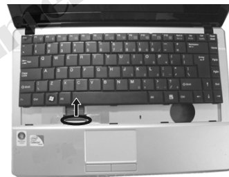
Figure 2-4 Disconnect the cable
