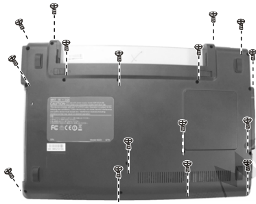
Figure 2-5 Remove the eighteen screws
