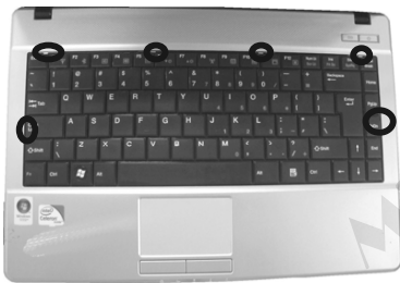
Figure 2-3 Loosen the six latches
