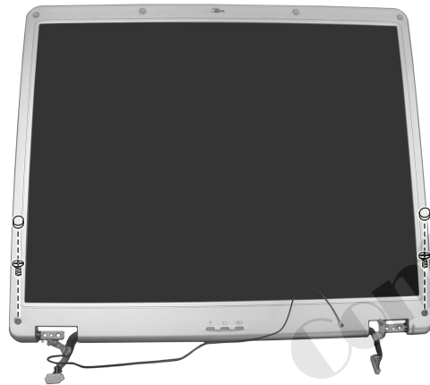
Figure 2-20 Remove LCD cover
