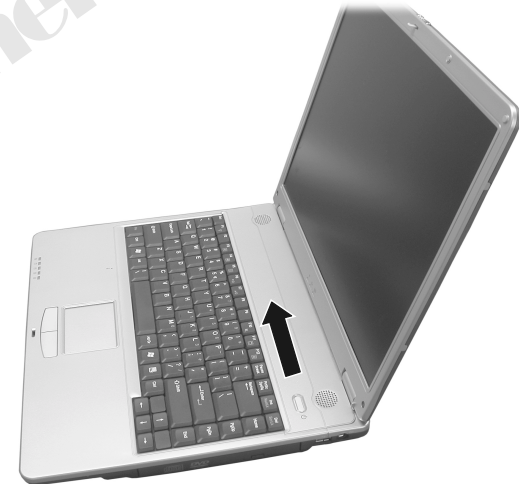
Figure 2-3 Lift the keyboard cover
