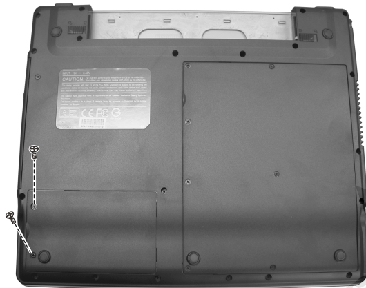
Figure 2-9 Remove the HDD compartment cover
