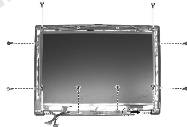
Figure 2-25 Remove ten screws and disconnect the cable
