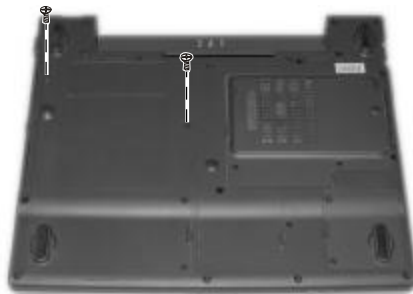
Figure 2-13 Remove two screws
