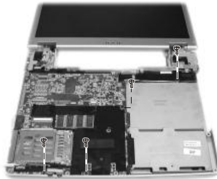
Figure 2-32 Remove four screws
