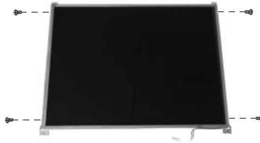
Figure 2-31 Free the LCD panel
