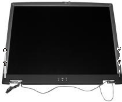
Figure 2-26 Remove LCD cover
