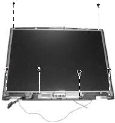
Figure 2-29 Remove the LCD panel
