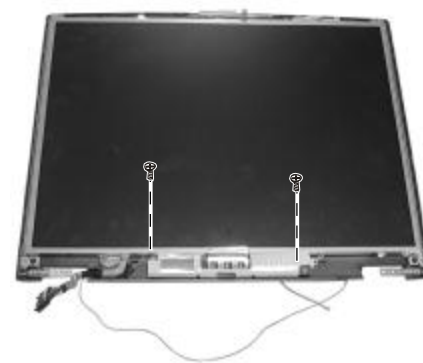
Figure 2-27 Remove the inverter board
