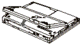
Figure 5-7 Latching the Notebook in the Detachable Bay
