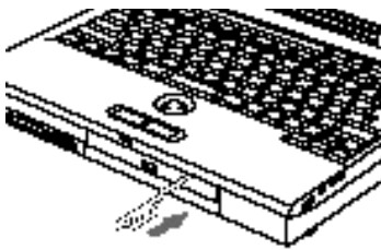
Figure 5-1 Emergency CD-ROM Tray Release
