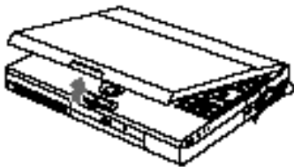
Figure 2-1 Opening the Display Panel
