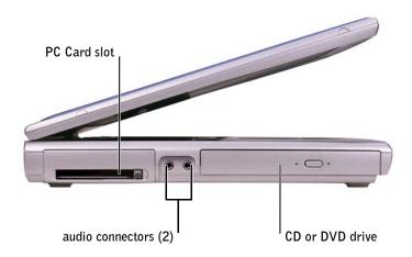
**PC CARD SLOT** — Supports one PC Card, such as a modem or network adapter. For more information, see "Using PC Cards" in the Tell Me How help file. To access the help file, see page 80.
