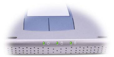
Turns on when you turn on the computer. Blinks or turns off in power management mode. Turns on when the computer reads or writes data. NOTICE: To avoid loss of data, never turn off the computer while the | light is flashing. 囝 Blinks to indicate battery charge status.
