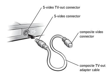
3 Plug one end of the composite video cable into the composite video connector on the composite TV-out adapter cable.
