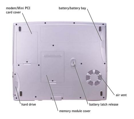
MODEM/MINI PCI CARD COVER — Covers the compartment that contains the modem and Mini PCI card. See page 102.
