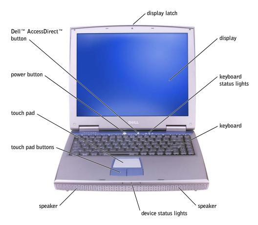
**DISPLAY LATCH** — Keeps the display closed.
