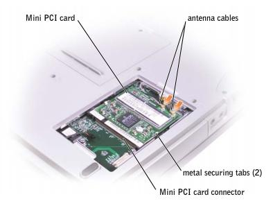
NOTICE: To avoid damaging the Mini PCI card, never place cables on top of or under the card.
