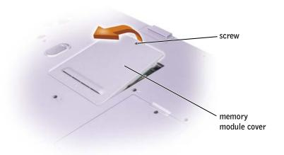
**3** Remove the screw labeled "O" next to the memory module cover.
