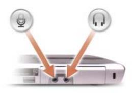
Attach a microphone to the  $\Theta$  connector.
