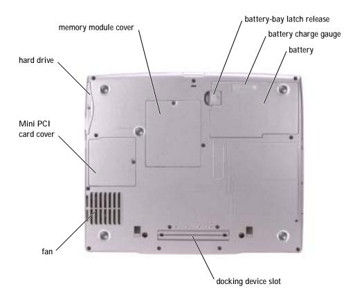
MEMORY MODULE COVER — Covers the compartment that contains the memory module(s). See "Adding Memory" on page 106.
