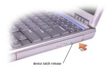
Pull the device by the latch release to remove the device from the module bay.
