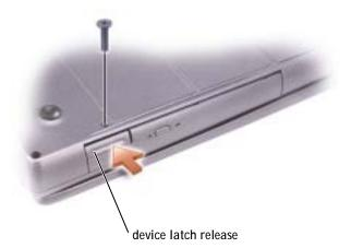
Press the device latch release so that the latch release pops out.
