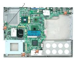
15. Remove the four hex screws on the back of the computer.
