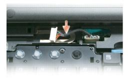
To replace the hinge cover, insert the left edge of the cover into the hinge cover slot, and press from left to right until the cover snaps into place.
