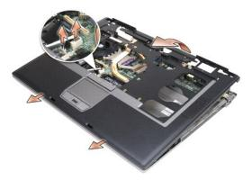
NOTICE: When replacing the palm rest, ensure the cable for the internal card with Bluetooth wireless technology is properly placed on top of the palm rest to avoid damaging the cable.
