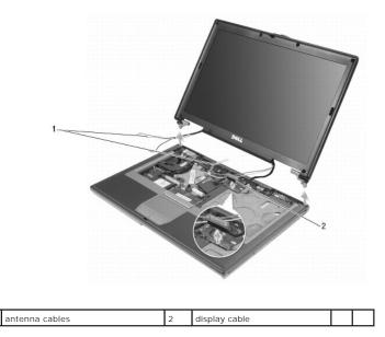
12. Lift the display assembly out of the computer base.
