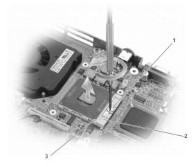
1 ZIF-socket cam screw 2 ZIF-socket 3 pin-1 corner of processor
