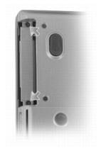
12. Remove the seven M2.5 x 8-mm screws from the bottom of the computer.
