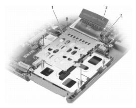
8. Use the pull-tab to disconnect the PC Card reader connector from the system board.
