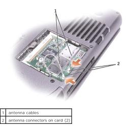
7. Lower the Mini PCI card toward the inner tabs to approximately a 20-degree angle.
