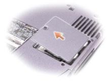
3. Place your finger under the cover at the indentation, and lift and slide the cover open.
