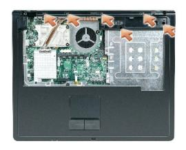
10. Disconnect the touch pad connector from the system board.
