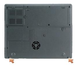
9. From the back of the computer, remove the two M2.5 x 8-mm screws labeled "D."
