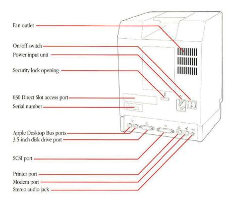
• 030 Direct Slot access port: Your 030 Direct Slot access port may look different from the one shown here, depending on the internal options installed in your system.
