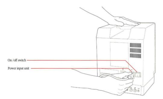
Plug the other end of the power cord into a three-hole, grounded outlet.
