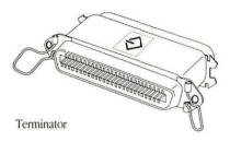
Devices connected to the SCSI port on the back of the main unit must have the proper number of **terminators** for the devices to work correctly and to prevent damage to the SCSI chip inside your computer.
