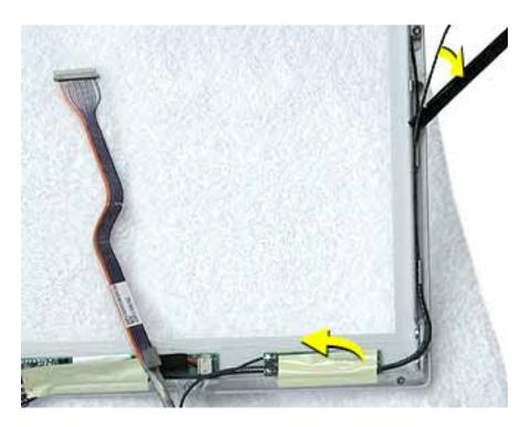
5. Warning: When removing the tape and spiral tube that bundles the microphone cable to the LCD cable, be careful not to strain or pinch the cables.
