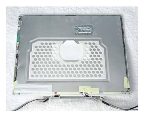
5. Peel up the tape if it covers the two screws at the clutch. Remove the two 11-mm long Phillips screw s.
