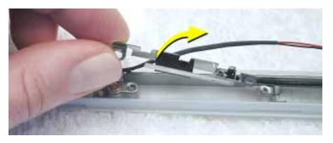
10. Unwrap the tape that secures the AirPort Card antenna to the cable bundle.
