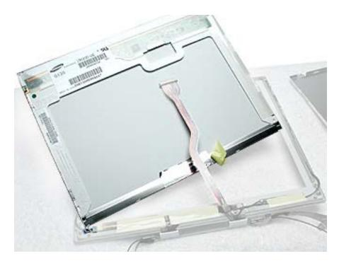
14. Disconnect the inverter cable from the inverter board at CN2 and remove the LCD panel.
