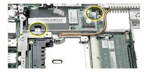
3. **Important:** Although the image below shows the LVDS cable removed, do not strain or remove the cable.
