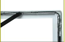
4. Free the microphone cable from the right corner of the bezel and from underneath the tape at the antenna board.
