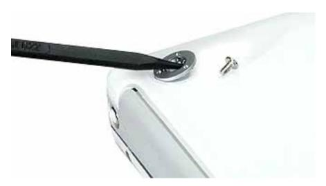
6. Remove the two Phillips screws next to the battery connector.
