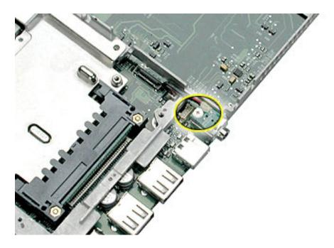
4. Remove the two screws holding the vent cover to the heat spreader.
