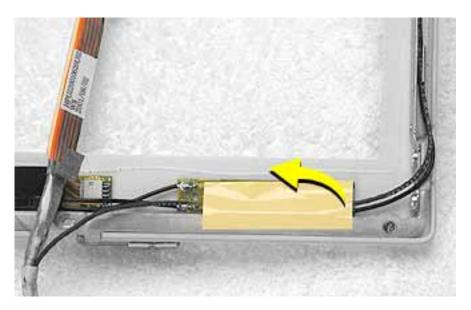
2. Note the placement of the antenna board and the routing of the cables that are soldered to and run along the bottom of the antenna board.
