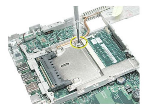
6. Tilt up the heat spreader and lift it off the logic board and out of the frame.
