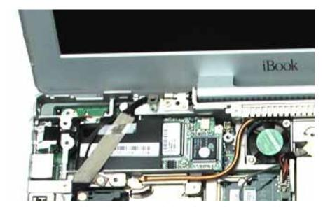
2. **Important:** Although the image below shows the LVDS cable removed, do not strain or remove the cable.
