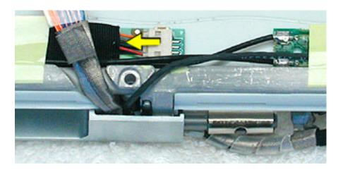
6. Remove the reed switch cable assembly.
