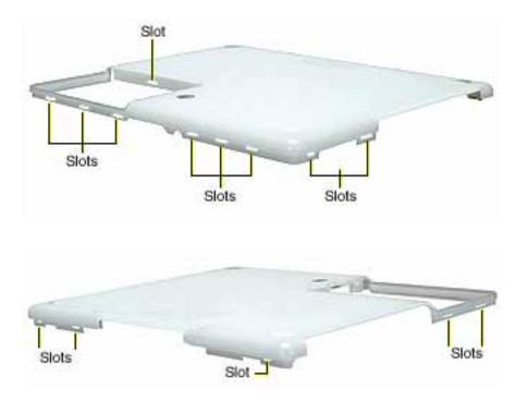
8. In the battery compartment, lift up the corner of the bottom case, and use a black stick to gently pry up the slot from the inner tabs on the frame.
