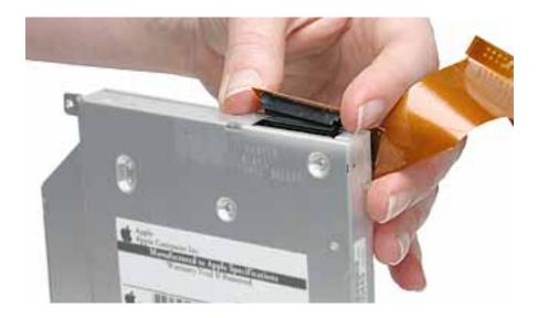
9. Remove the two screws that hold the mounting bracket to the optical drive.
