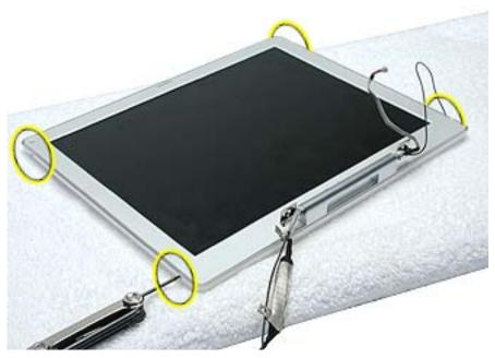
2. Using a black stick, pry up the bezel from the display housing. Carefully work the black stick around the outer perimeter and corners of the bezel.
