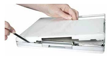
12. If you are replacing any additional parts at this time, remove the two springs from the battery compartment so they do not fall out and get lost.
